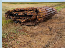
BF#8272 The old culvert was badly corroded.
